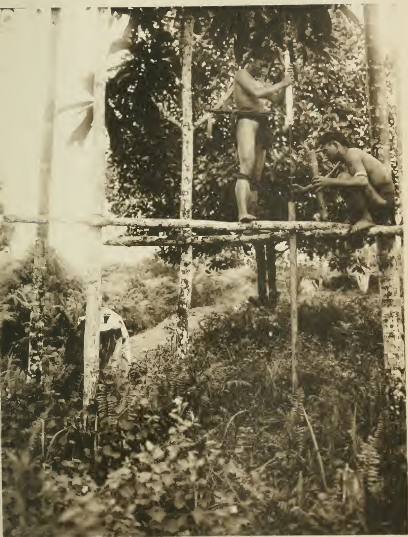
PLATE 113. KENYAHS DRILLING A BLOW-PIPE.
