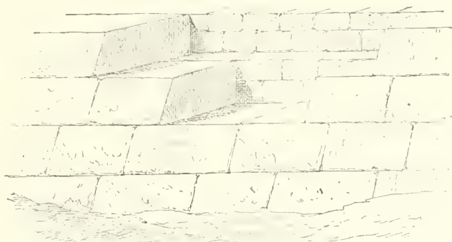
FIG. 155 —The casing of the pyramids; drawn in perspective from the elevation of Perring.
