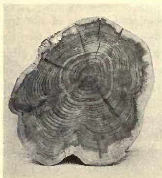
FIG. 69. Transverse section of yew, showing annual rings. Longest diameter, 5\frac{1}{2} "; shortest, 4\frac{1}{3} "; number of rings, 51. It will be noticed that the section is excentric; this is due to irregular growth. The light coloured, outer zone, is the alburnum, or sap-wood; the dark, inner zone, the duramen, or heart-wood. The large, radial cracks are the results of shrinkage. These cracks run along the lines of the medullary rays, though the actual rays are much too fine to be seen without a good lens. (For an excellent description of such a section, see G. S. Boulger, Wood , 2nd edition, 1908, p. 301.)
