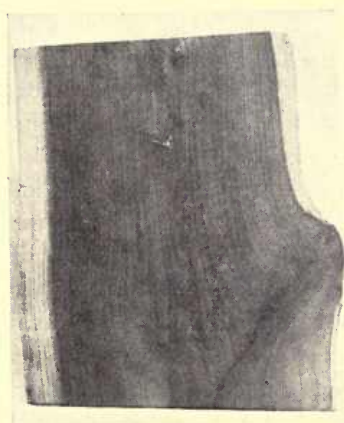
FIG. 70. Longitudinal, tangential section of yew. In this section, taken with the "grain," the annual rings appear as alternate parallel strips of dark and light wood. The tracheids, or elongated thick-walled cells, are invisible to the unaided eye.
